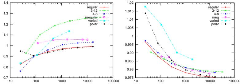
Figure 5: Left: uniformly loaded linearized plate test for different mesh types. Right: Sphere recovery test. The maximal computed pointwise displacement is shown relative to the maximal pointwise displacement for the analytic solution.
